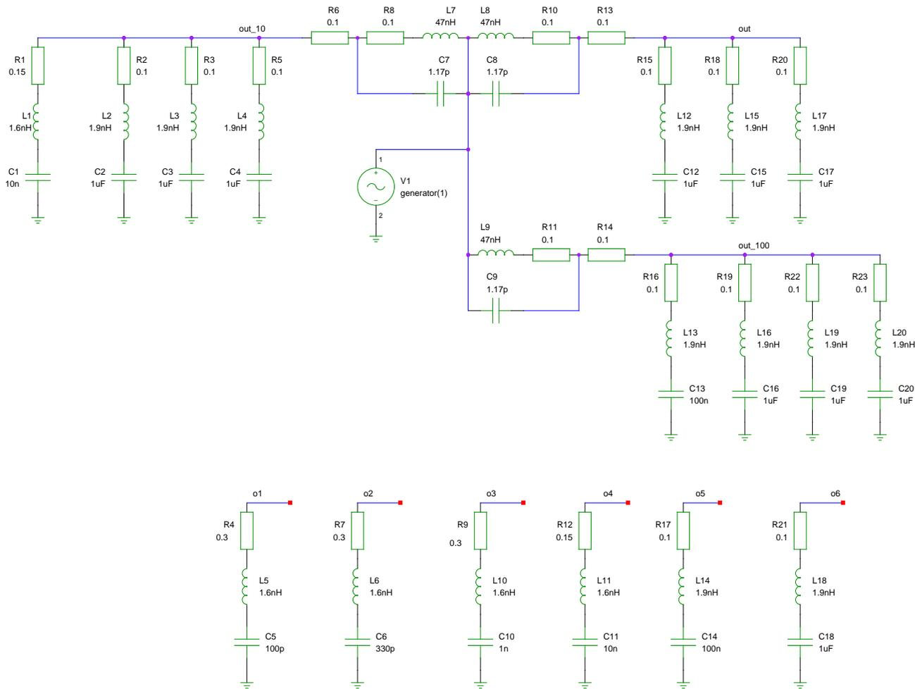
A5 Gnuicap directive .print ac vmdb(out) vmdb(out\_10) vmdb(out\_100)
